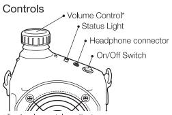
\* Turn the volume control cap with extra care. **Stop turning** when the knob reaches both ends.
