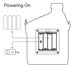
Plug in Boombottle Lite into a USB power supply or insert 4 AA rechargable batteries, following the indicated + & - direction. Then press the switch to On.
